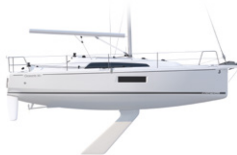
PROFILE Lifting keel version - Quille relevable
